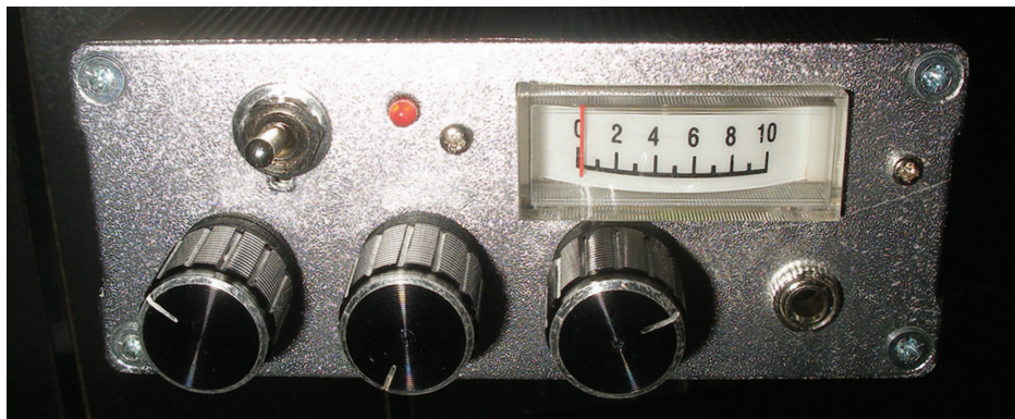
PHOTO 1: The modified kit with an edge meter. Left to right: Tune, Squelch, Volume and headphone socket.
